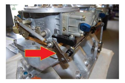
4. Tighten the screws on both the arms and locking collars. <u>\*\*\*Caution it is not necessary to overly</u> <u>tighten these screws as the serrations prevent the arms from slipping\*\*\*</u>
