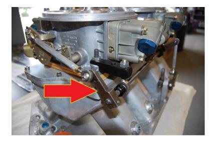
4. Tighten the screws on both the arms and locking collars. \*\*\*Caution it is not necessary to overly tighten these screws as the serrations prevent the arms from slipping\*\*\*
