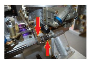
3. Slide on first the other locking collar with set screw, and then a serrated arm onto the front of the serrated shaft. The front arm should line up fairly close perpendicular with the rear arm.
