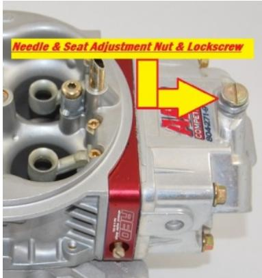
If you want to *raise* the level, gently loosen the nut about a  $\frac{1}{2}$  turn and re-tighten the lock screw. Re-check the level and repeat as needed. If you want to *lower* the level, you will need to loosen the nut slightly to break the lock screw loose, then tighten the nut a  $\frac{1}{2}$  turn and re-tighten the lock screw and repeat as needed. Be sure you hold the lock screw still as you tighten the nut to ensure the float height will change accordingly.
