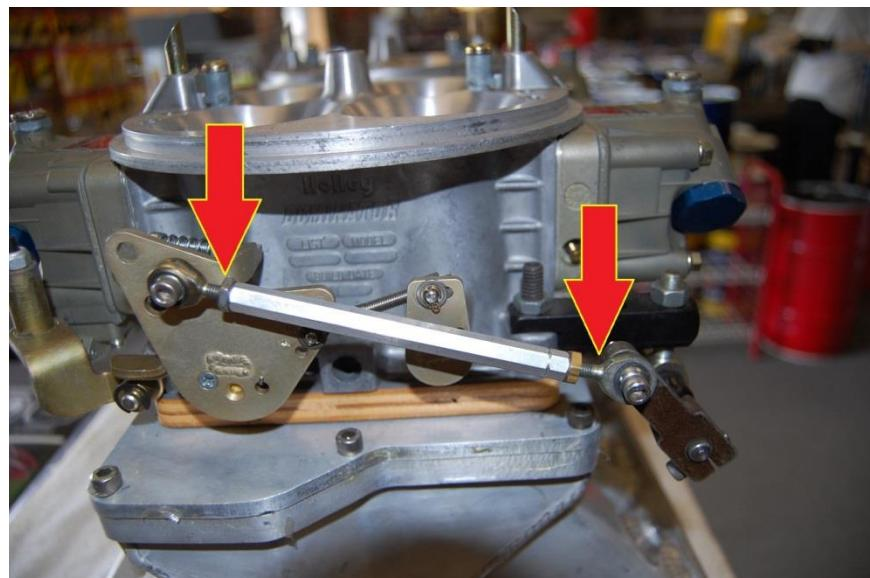
6. Enclosed with the linkage kit are two different types of carburetor arm spacers. One series of carburetor arms has a 3/16" hole and one has a 1/4" hole. The spacers for the 1/4" holes have a turned down portion which fits into the carburetor arm. The 3/16" spacers are a straight spacer. Select the spacers that fit your carburetor and install the other end of the linkage onto the carburetor using the 10-24x7/8" bolts and lock nuts.
