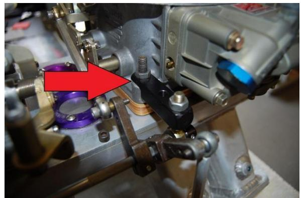
2. Slide the serrated shaft thru the front spherical rod end with the long serrations toward the rear carburetor. Next slide on one of the locking collars with set screw. Slide in two serrated arms facing toward the front of the vehicle. Position the arms slightly less than 90 degrees from each other. Slide the serrated shaft into the rear spherical rod end.
